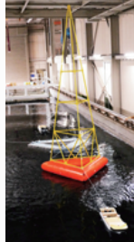
Experiment on a floating transmission tower for offshore overhead power transmission
