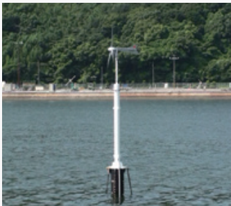
1/10 model experiment of 2-MW real turbine
